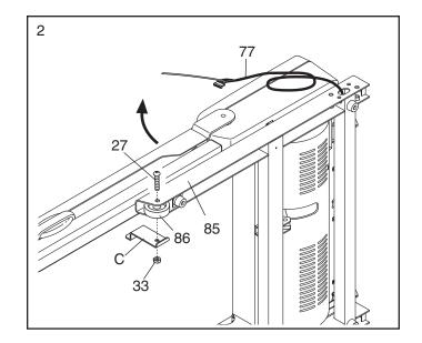
Identify the Right Upright (78) and the Right Upright Spacer (80), which are marked with stickers. Insert the Upright Wire (77) through the Right Upright Spacer as shown.
